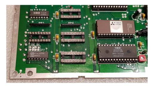
**STEP09** – Insert the 64k ram daughter board to the right place. The gold pins can be bent easily, care must be taken with them. Also install the 64k ram ICs to the 2x9 pin sockets. Pay attention to the polarity!
