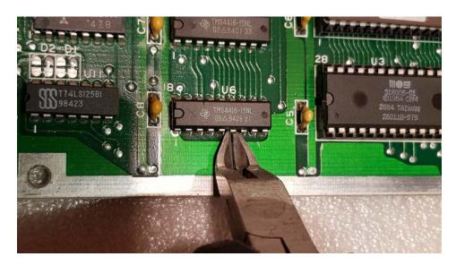
**STEP04** – Remove the ICs with a flat head screwdriver. These parts are damaged, but don't worry about, we will not need it.
