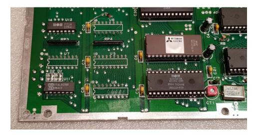
**STEP06** – With a desoldering braid carefully remove the legs and the tin solder from the holes. One by one... Use a wide clip if needed.
