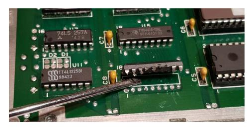
**STEP05** – Remove completely the parts from the mainboard.
