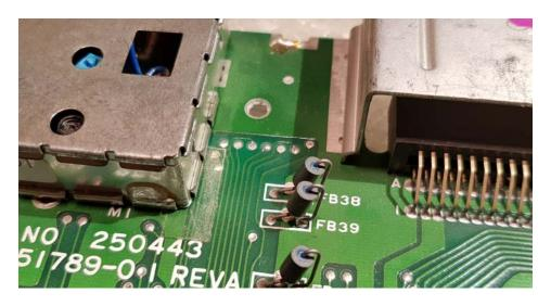
**STEP11** – Need a desoldering braid again. Remove the tin solder from the left two holes (both sides).
