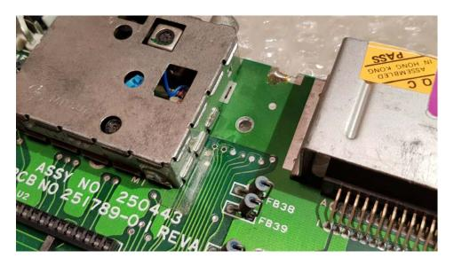
**STEP12** – Insert the two pins connector and solder iron to the mainboard.
