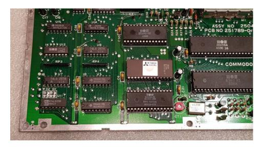
**STEP03** – Carefully cut the legs of the U5, U6, U7, U8 with an oblique nippers.
