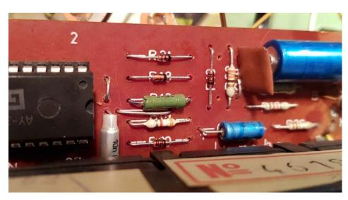
**STEP06** – Narrow and remove the next parts from the mainboard: the R17 resistor and C22 electrolytic capacitor.
