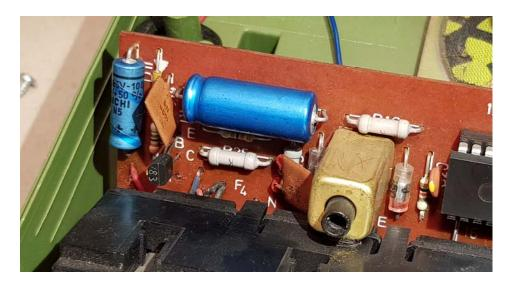
STEP10 – Solder iron the pins to the remaining wires. Its red, white and 2x black. The red is the 9V (P3), the white is the composite video out (V1), and the blacks are the grounds (F3 and F4).
