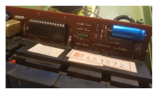
STEP08 – Turn on the mainboard. Insert the small trimmer potentiometer to the R17 resistor place and solder iron to the vias. Use again the schematics if needed from STEP05.
