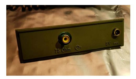
STEP13 – Install the pcb with the tiny panel to the pong. Be carefully cause no more enough space here. A good trick about loosen the screw or screws between the pcb and the tiny panel until not slide to the right place.
